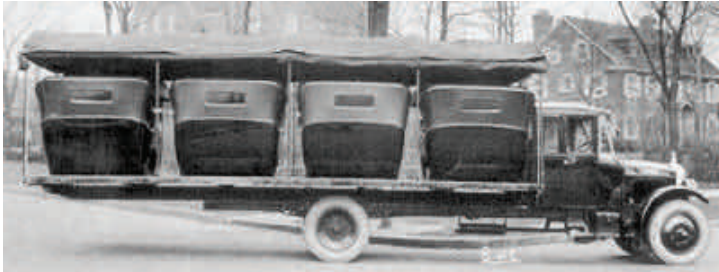
Gotfredson truck built specifically to transport auto bodies to and from the American Auto Trimming plant in Canada.
